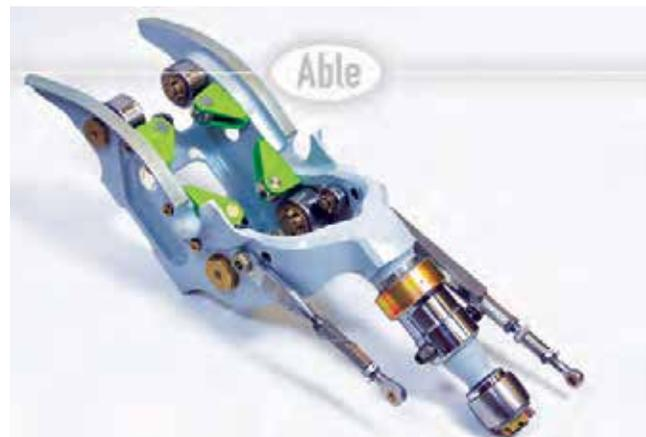
Complex mechanical assemblies, such as this 737 flap carriage, lend themselves to refurbishment using DER repairs, according to Able Aerospace. Able photo.
