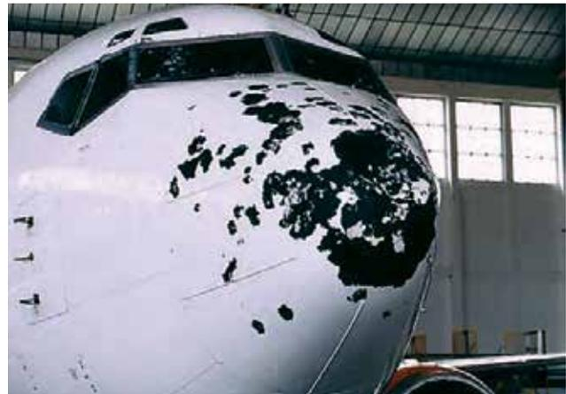
DER Associates, a consulting DER firm, says it has worked with a wide range of fixed- and rotary-wing aircraft, repairing planes with everything from bullet holes to softball-sized hail damage, like the one shown here. DER Associates image.
